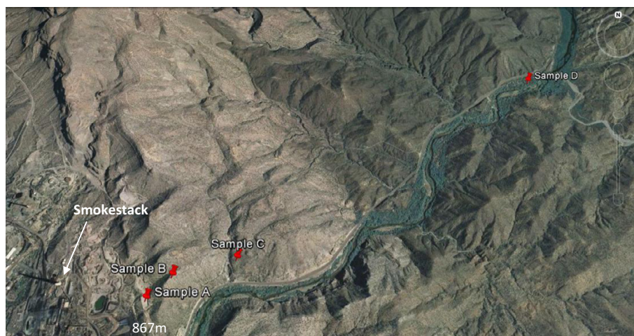
Fig. 3. Satellite picture showing the four soil sampling locations (labeled A–D) at the Hayden site. The shadow of the 305 m high smokestack can be seen towards the WNW. Approximate distances of the sampling points from the smelter location: A – 650 m, B – 900 m, C – 1300 m, and D – 4000 m. Altitudes with respect to sea level of sampling points are: A – 680 m, B – 760 m, C – 710 m, and D – 620 m. Source: Google Earth.
